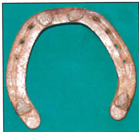
These borium spots are too big, uneven, and too far out on the edge of the toe
